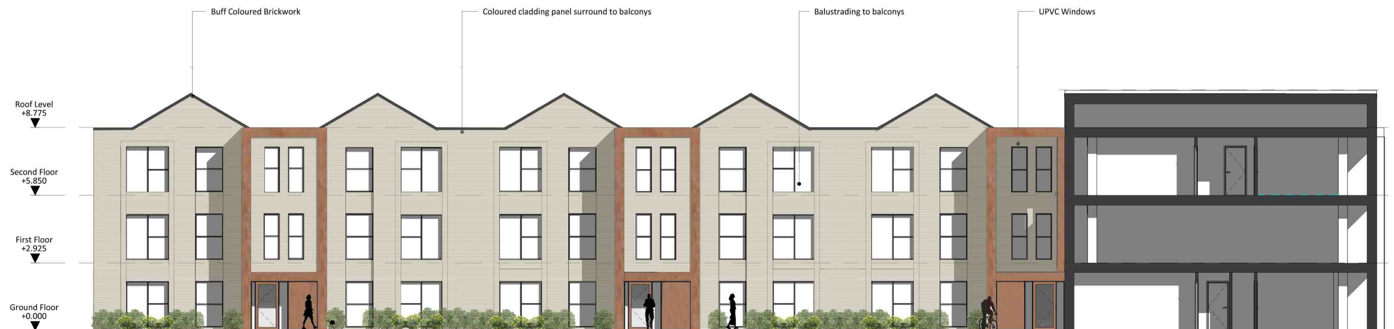
2. Proposed Car Park Elevation SCALE - 1 : 100@A1
